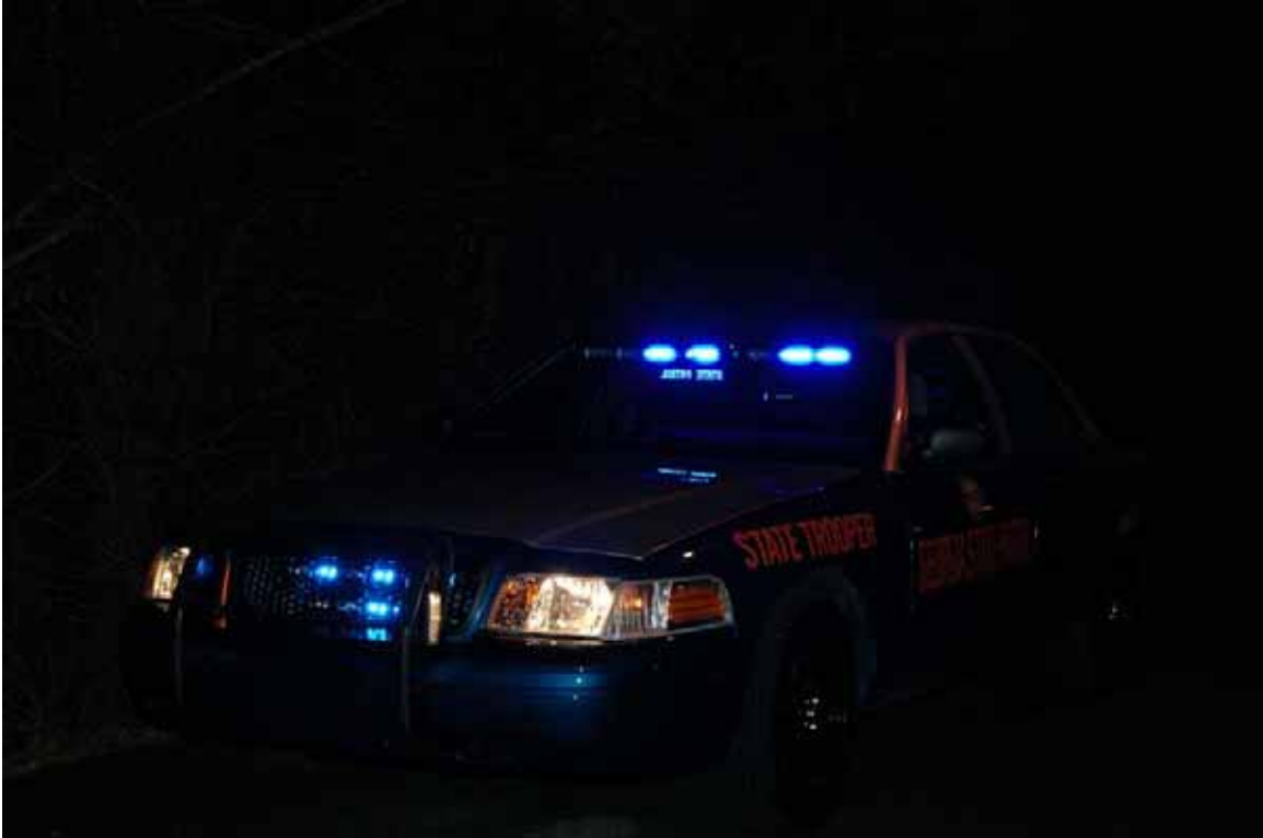
Slick top Georgia State Patrol car equipped with illuminating agency identifier.
